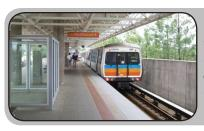
**HRT** operates on electric railway with high speeds, rapid acceleration of passenger rail cars, high platform loading, and grade separated, exclusive rights-of-way
